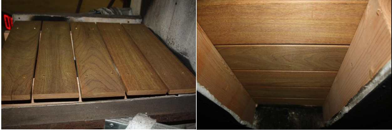
Figure 3. Representative test assembly for under deck tests.
